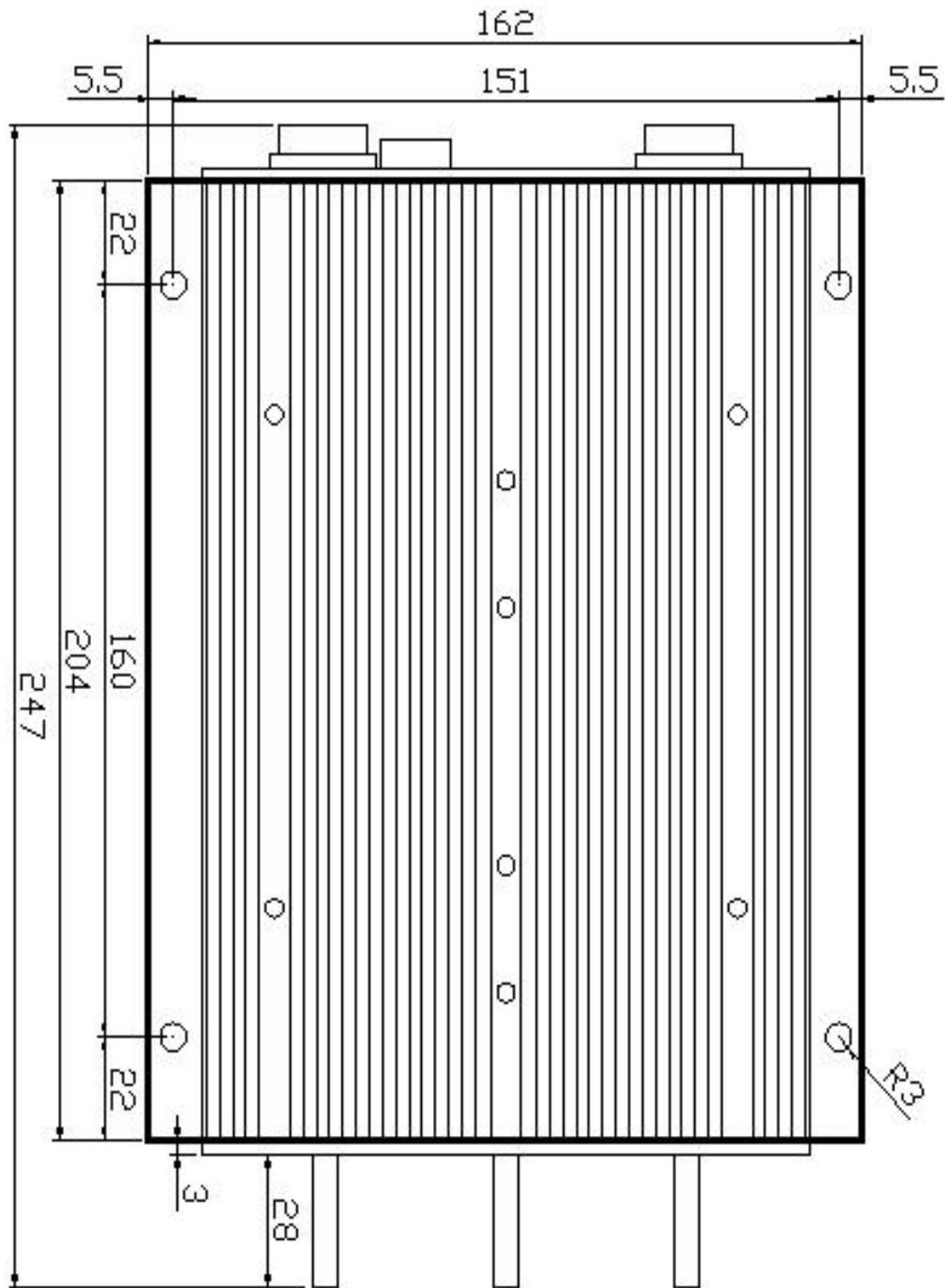
**Figure 1:** Height: 84 millimeters
