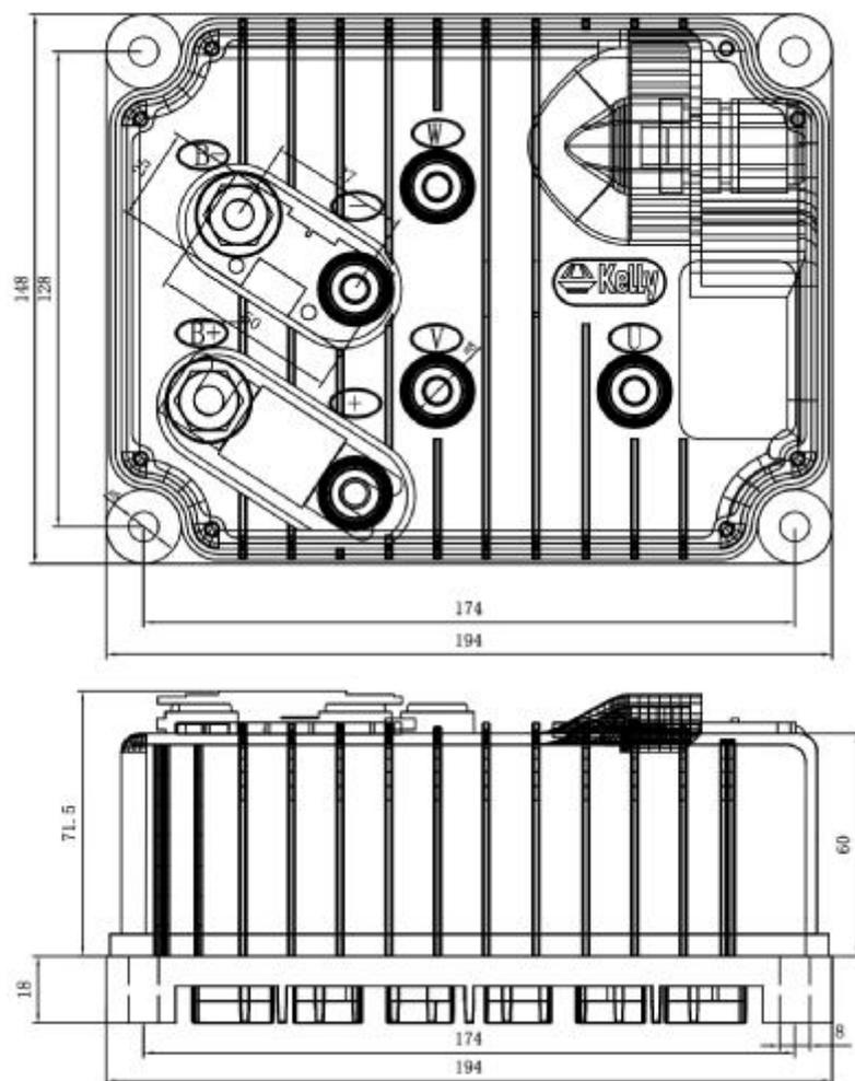
Figure 1:KLS-D mounting holes' dimensions (dimensions in millimeters)
