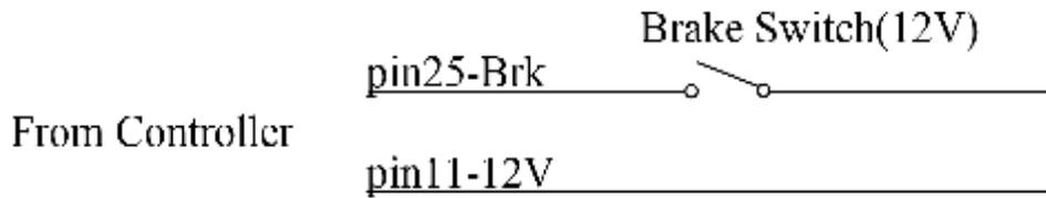
**Figure 6:** Wiring of brake switch(12V): 12V is provided by KLS-D controller on pin11
