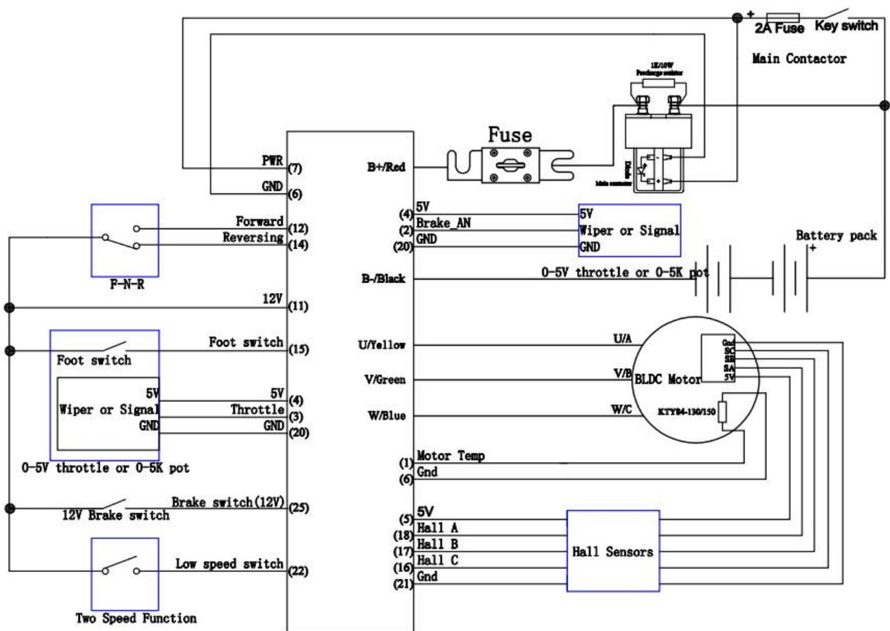
**Figure 3: KLS-D controller standard wiring(F-N-R Control)**
