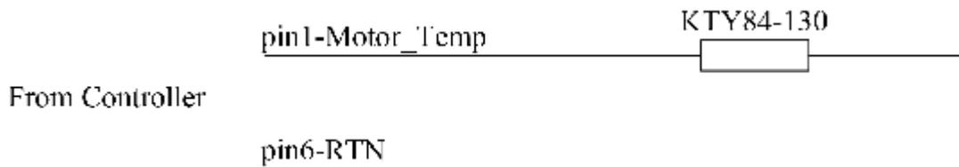
**Figure 7: Wiring diagram for motor temperature sensor**
