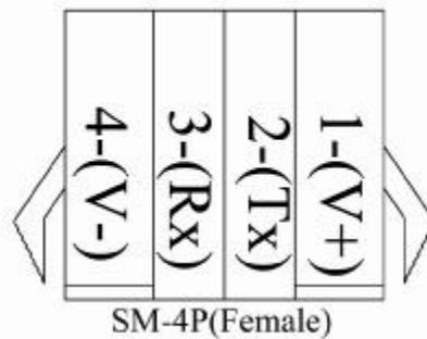
**Figure 9:** SM-4P connector for communication interface on KLS-D controller
