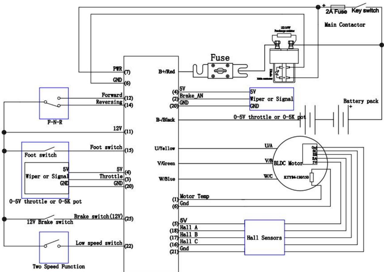
**Figure 3: KLS-D controller standard wiring(F-N-R Control)**
