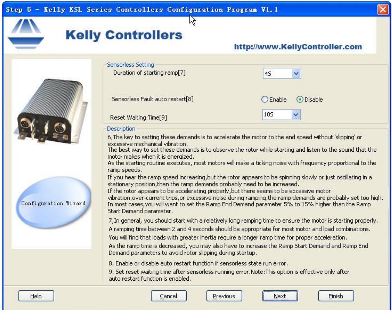
(7).Duration of Starting Ramp. In general, you should start with a relatively long ramping time to ensure the motor is starting properly. A ramping time between 2 and 4 seconds should be appropriate for most motor and load combinations. You will find that loads with greater inertia require a longer ramp time for proper acceleration. As the ramp time is decreased, you may also have to increase the Ramp Start Demand and Ramp End Demand parameters to avoid rotor slipping during startup.
